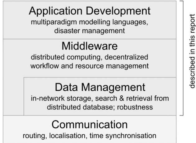
Figure 2: Logical layers of our system architecture.
